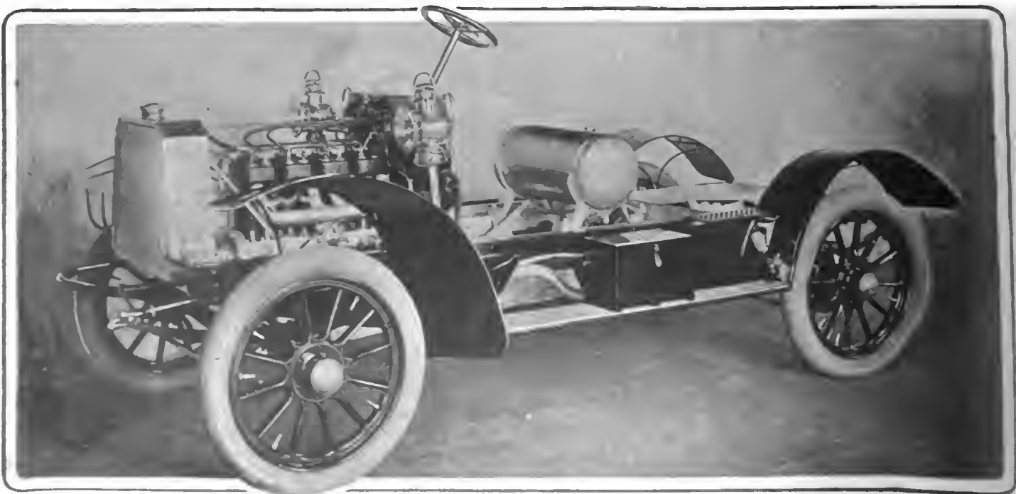
CHASSIS OF GROUT FOUR-CYLINDER GASOLINE TOURING CAR EXHIBITED AT THE BOSTON SHOW.
